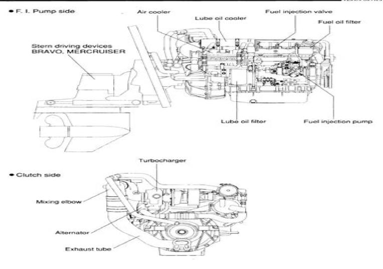
[Note] Above drawings show the 4LHA HTZE/HTZP engines.
