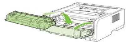
If no paper was jammed inside the print-cartridge door, open the jam-release door at the back of the product.
