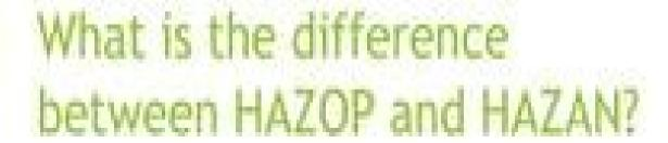
The main goal of HAZAN is to provide the best selection of means of controlling or eliminating the risk. A hazard and operability (HAZOP) study is a design review technique used for hazard identification, and for the identification of design deficiencies which may give rise to operability problems.
