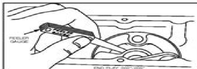
Fig. 893 – CHECKING CRANKSHAFT END PLAY
