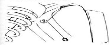
Loosen the screws ③ and remove the right frame cover.
