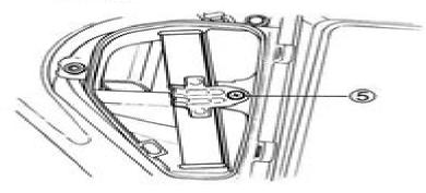
Loosen the screw ⑤ and remove the air cleaner element.
