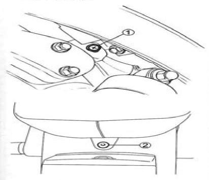
Loosen the screws ① (right and left) and the bolt ②, and remove the seat.
