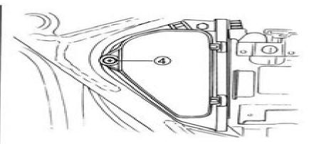
Loosen the screw @ and remove the air cleaner case cover.
