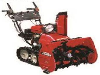
Horda's infinitely variable Hydrostatic transmission makes & easy to find the right speed for any snow cleaning skustion and operator preference. A single lover accurately adjusts ground speed without affecting auger ratation speed.
