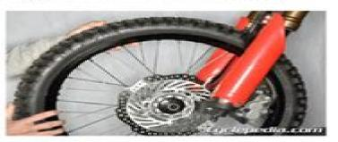
Roll the wheel forward and out from between the forks. Do not apply the brake when the disc is not between the pads.
