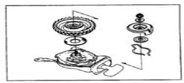
Pull the starter rope slowly and check the operation of the starter gear and return of the rope.
