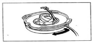
3) Wedge the end of the rope in the notch on the edge of the reel and install the reel aligning the groove in the reel with the spring end.
