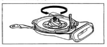
5) Pass the rope end through the hole out of the starter case by holding the starter reel. Insert the rope into the starter grip and tie the rope end and install the grip cap:
