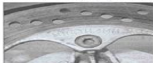
8.3 The minimum disc thickness is marked on each disc
