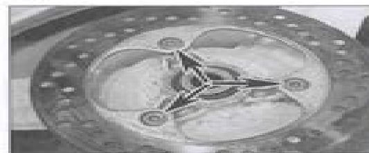
8.5a The disc is secured by three bolts (arrowed) on J and K models . . .
