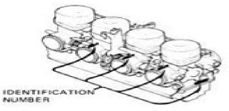
The carburetor identification number is on the carburetor body left side.
