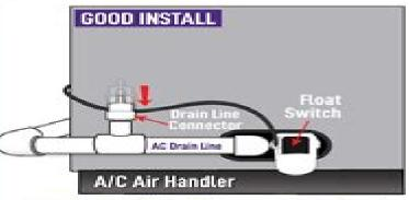
OPEN DRAIN LINE - Remove Drain Cap from Access Point & place Drain Line Connector over open line.
