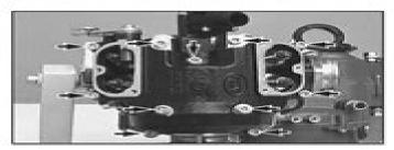
Remove all 11 bolts. Then remove the cylinder head top section.
