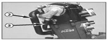
Undo the 4 hose clamps and remove both hoses (@ and @)...
