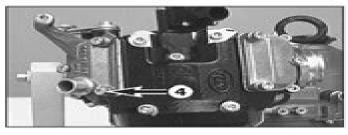
Remove all 6 bolts • together with the seal rings and take off both valve covers together with the gaskets.
